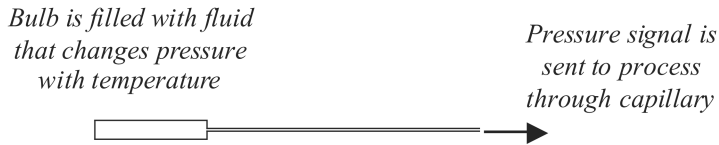
FIGURE 5.1.15 Schematic of a bulb and capillary sensor.
