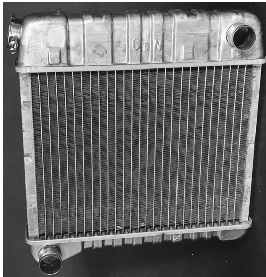
a. A 1980 Chevette radiator. Cross-flow exchanger with neither flow mixed. Edges of flat vertical tubes can be seen.
