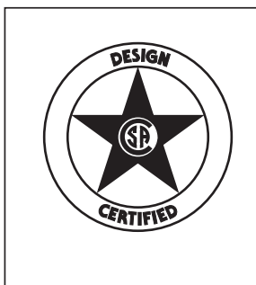
3-20. These symbols of the Canadian Standards Association certifies the safety of gas-fired equipment. The symbol above certifies that the equipment complies to ANSI Standards for The United States. The symbol to the right certifies that the equipment is approved for use in Canada.
