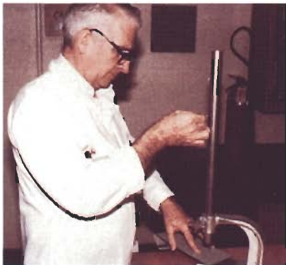
American Standard engineers test powder paint for impact resistance so the paint will stay intact even if the metal gets dented.
