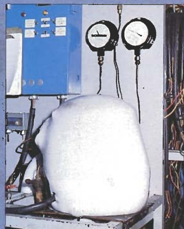
"Snowball" has been undergoing a continuous flood back test in our compressor life test facility since 1973. The test demonstrates the reliability of the compressor under conditions like low indoor airflow or system overcharge.
