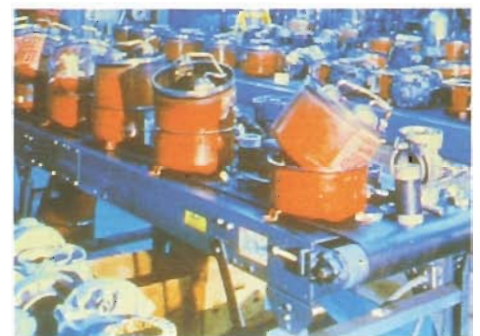
Every time a Duration compressor is returned from the field, it's cut apart and analyzed in order to identify any possible failure trends.
