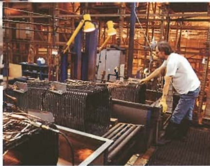
Each American Standard unit is given a complete run test at the end of the line. Air conditioners are given 32 checks; heat pumps, 64.
