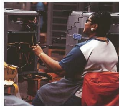
Each brazed joint is carefully checked multiple times during the manufacturing process.
