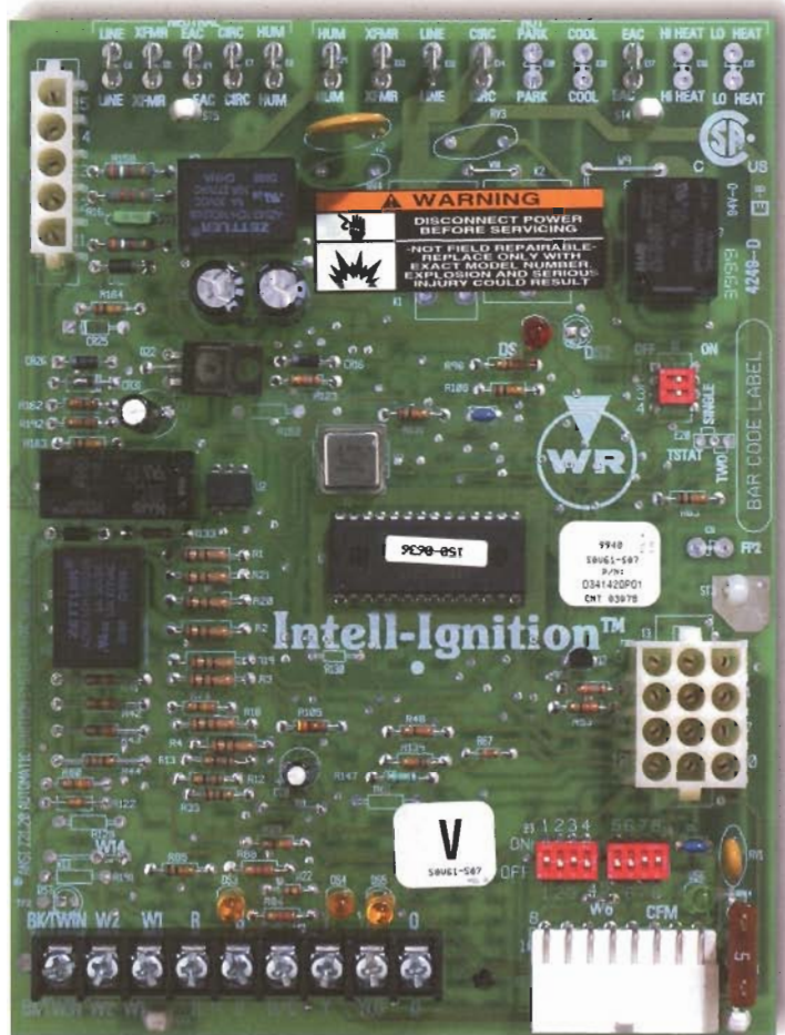
American Standard uses integral furnace controllers on all Freedom furnace models. The board pictured here is on the Variable Speed Freedom 80.
