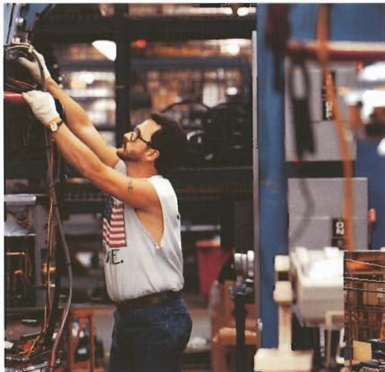
Each American Standard unit is given a complete run test at the end of the line. Air conditioners are given 32 checks; heat pumps, 64.
