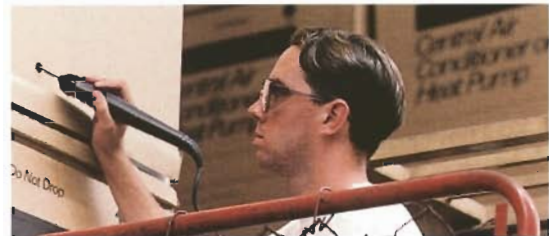
Each unit gets its last leak test in the warehouse where the operator inserts a leak detector in a small hole in the unit carton. If a leak is found, the unit is sent back to be reworked.
