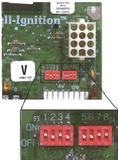
American Standard's variable speed products feature a controller that allows the installer to program in the right CFM by setting dip switches.
