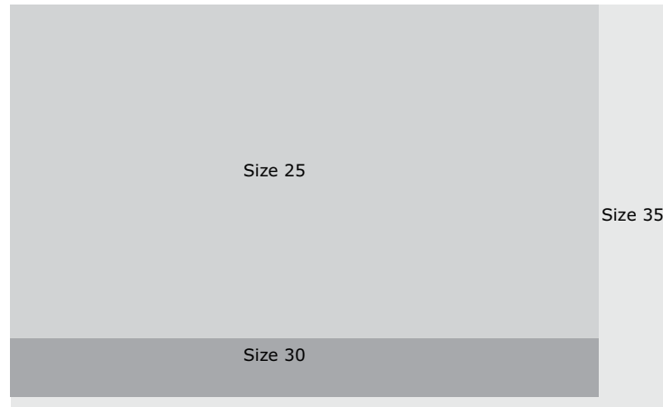
Figure 11. Impact of coil face velocity on AHU footprint (see Table 4)
