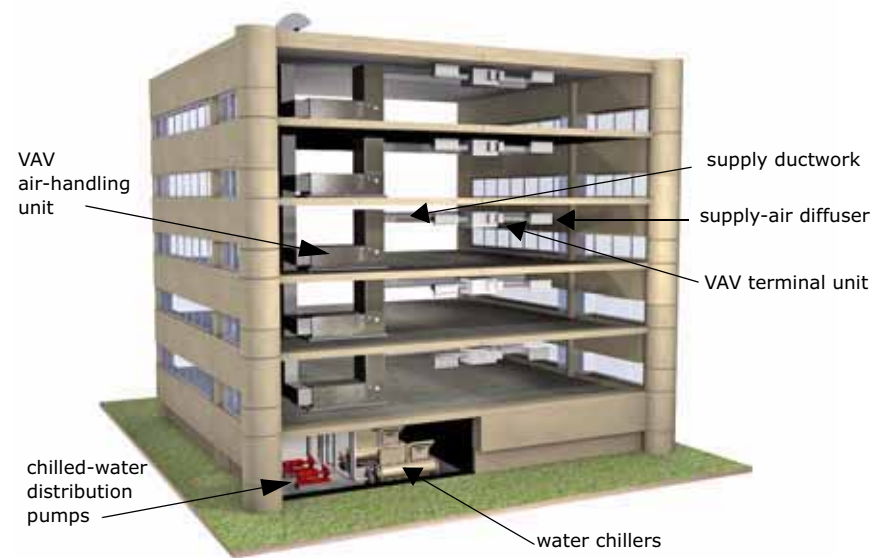
Figure 1. Primary components of a chilled-water VAV system
