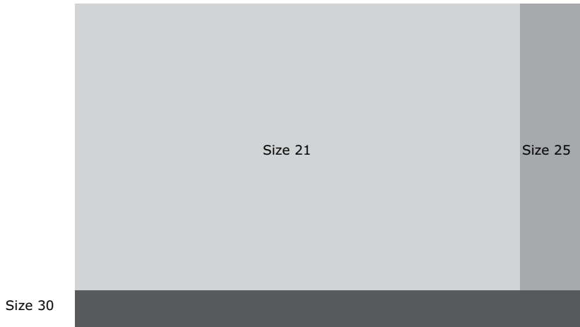
Figure 105. Impact of cold-air distribution on AHU footprint (plan view)
