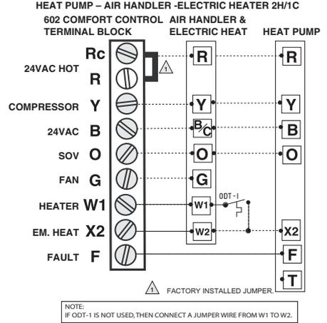
In Installer Setup, set system type to **2Heat/1Cool Heat Pump**.
