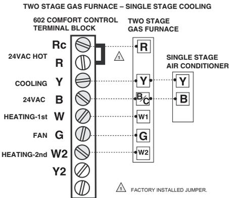
In Installer Setup, set system type to **2Heat/1Cool Conventional**.
