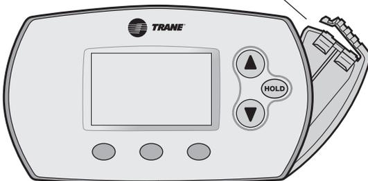
Insert fresh AA alkaline batteries, then reinstall battery holder
