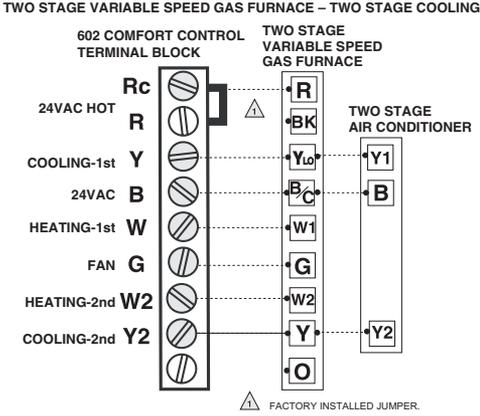
In Installer Setup, set system type to **2Heat/2Cool Conventional**.
