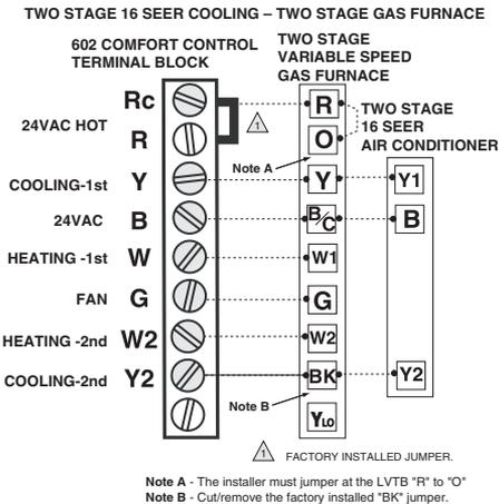
In Installer Setup, set system type to **2Heat/2Cool Conventional**.
