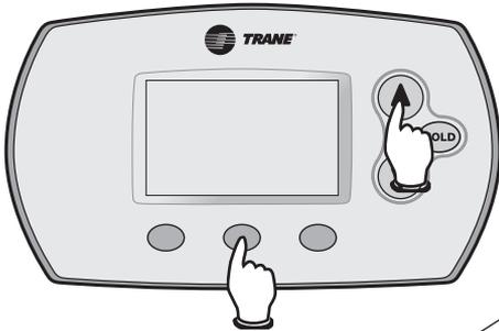
To begin, press and hold the ▲ and FAN buttons until the display changes
