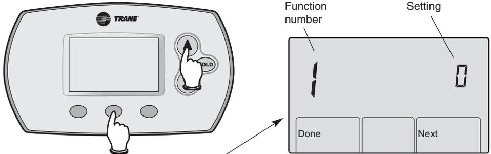
To begin, press and hold the ▲ and FAN buttons until the display changes
